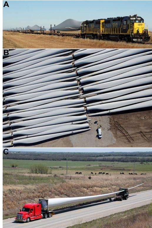
Figure 5. Railroad logistics and truck transportation of turbine blades in Kansas. A – turbine blades on the K&O Railroad wait for unloading at a storage area near Larned. B – vertical view of turbine blades stored in the BNSF Railway depot at Emporia. Service truck provides scale; kite photograph by JSA with D. Leiker. C – turbine blade transported by truck on state highway 99, Elk County. These blades are typically about 50-60 m long.
