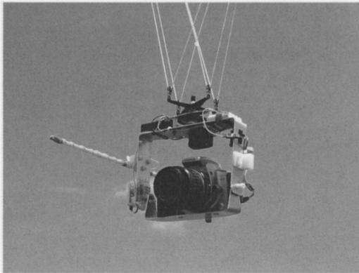
Figure 3. *Canon Digital Rebel* camera rig for kite or blimp aerial photography. The six-megapixel SLR camera is radio-controlled from the ground. It can pan (0-360°) and tilt (0-90°) to provide views in all orientations relative to the study site. Camera rig built by Brooks Leffler.
